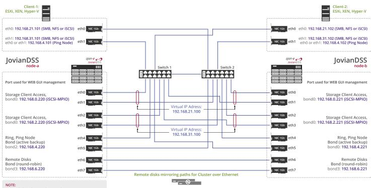
Ring path (heartbeat) and Ping nodes must run on Active-Backup bonding. Ring and Ping IP must be configured in the same network subnet.
